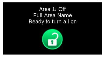
The Main icon serves as both an indicator of the arming state and alarms, and as an icon to press to change the arming state. The text above the icon provides instructions.
